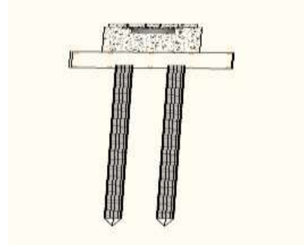
Gambar 5.12 Pondasi Bore Pile
