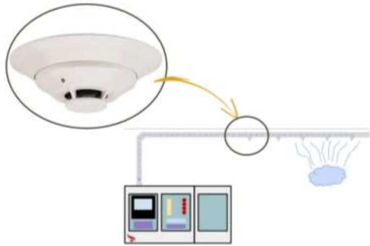
Gambar 5. 63 Sistem smoke detector.
