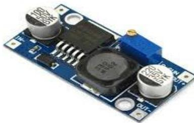
Gambar 2.4 Modul *Step Down DC Buck Converter* LM2596
