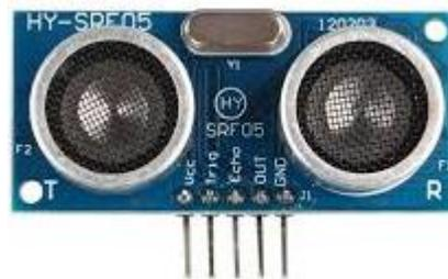
Gambar 2.2 Sensor Ultrasonik SRF-05
