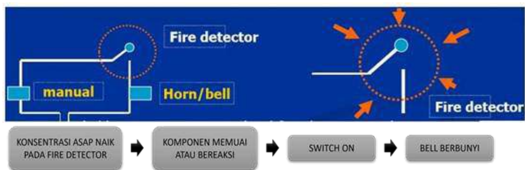
Gambar 4. 8 Prinsip Kerja Alarm System Sumber : Google 2023
