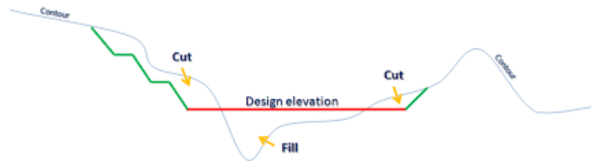
Gambar 4.2 Metode Cut And Fill Sumber : Firtolab
