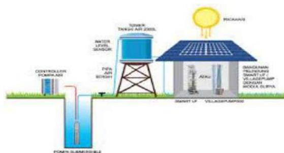
Gambar 5. 47 Sistem Down Feed
