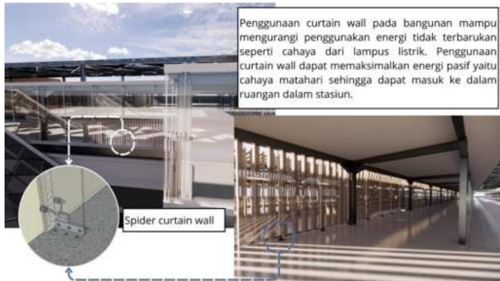
Gambar 5. 26 Konsep Material Dinding Curtain Wall
